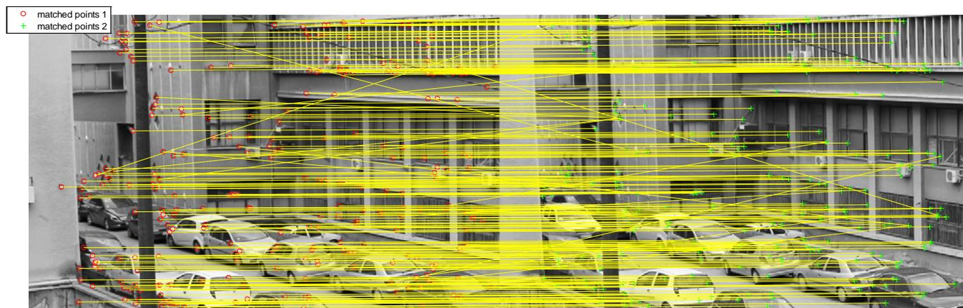
Fig. 10. Matched MSER/SURF features of original and shifted image used for feature-based image alignment. Note that there are some false detections, but that most of them are correct.
