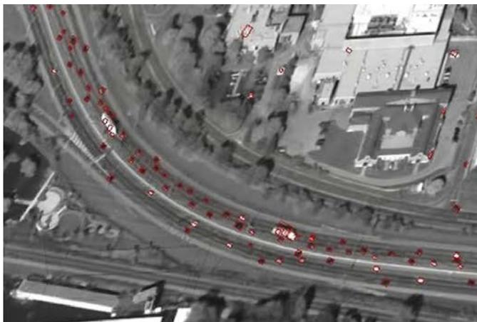
Fig. 8. Wide area motion imagery frame example. Red circles represent detected maximally stable extremal regions which refer to vehicles. Example is taken from [5].
